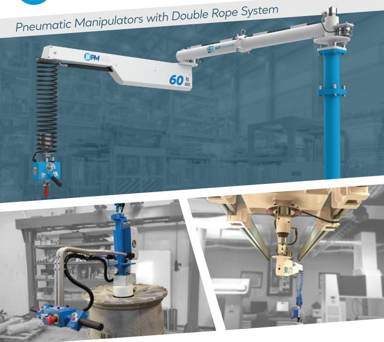
**BPM Supporter Double Rope Manipulators** are designed for **ergonomic**, **safe**, and **efficient material handling** in industrial environments. The load is guided to the balancing unit via **two independent steel ropes**, enabling a **weightless working experience**.
